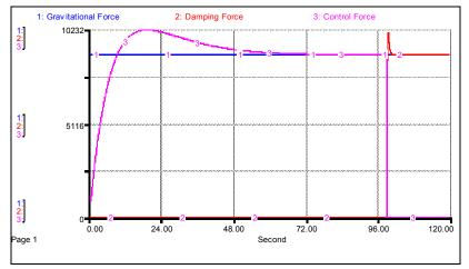
Figure 6: Absolute values of the forces acting on the vehicle during landing<sup>4</sup>
