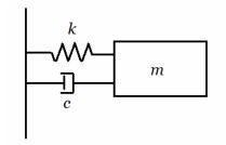
Figure 7: Mass spring damper schematic
