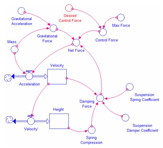
Figure 2: Stock-flow diagram of the model
