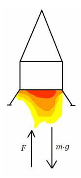
Figure 1: Free body diagram of the vehicle with a control force (F) generated by the reverse force thruster and the gravitational force  $(m \cdot g)$
